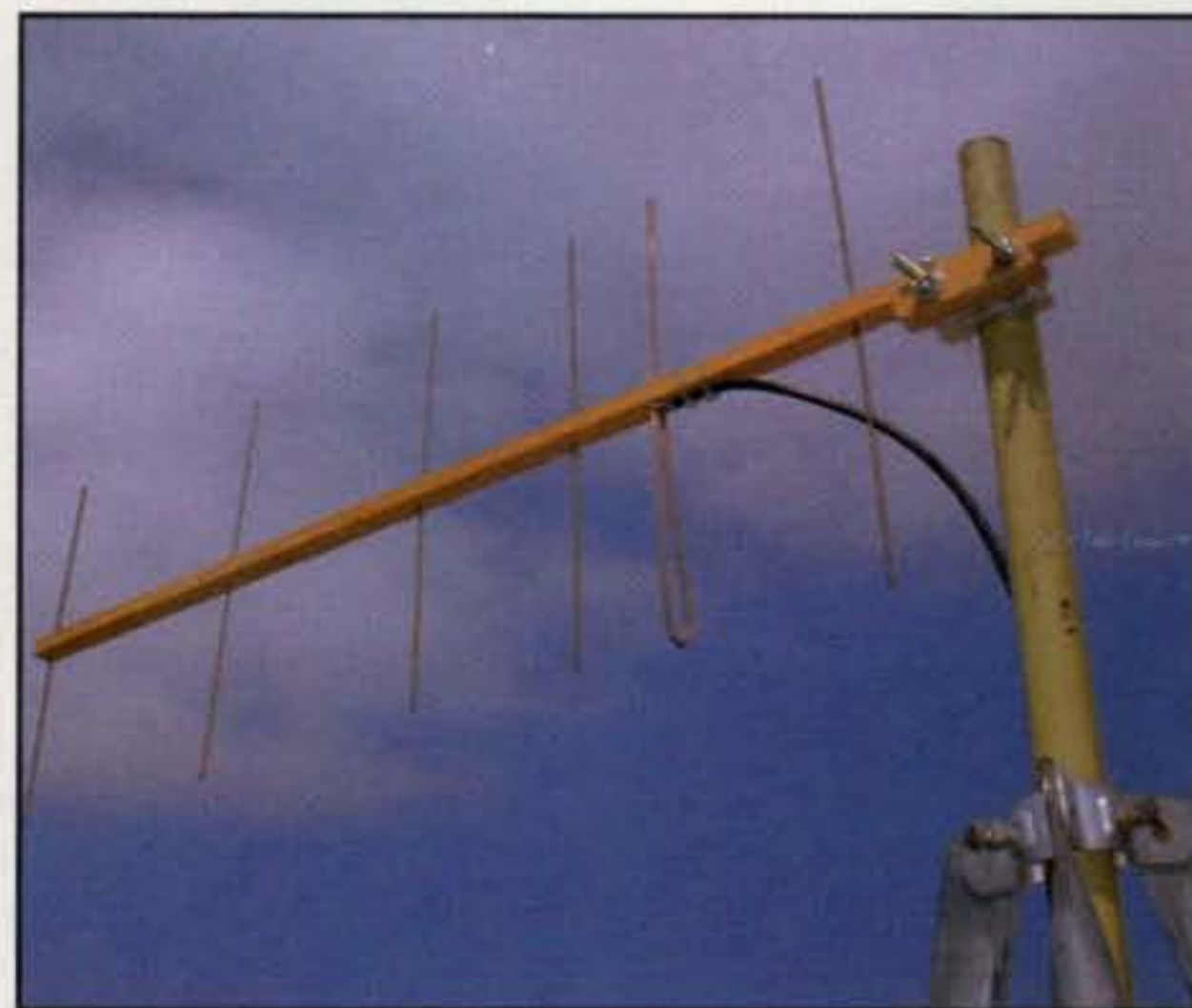
Photo A—An ATV Cheap Yagi. This antenna will cover the two popular amateur television channels at the lower end of the 70-cm band.
